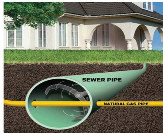
Router Ready to Cut a Cross-Bored Gas Pipe
